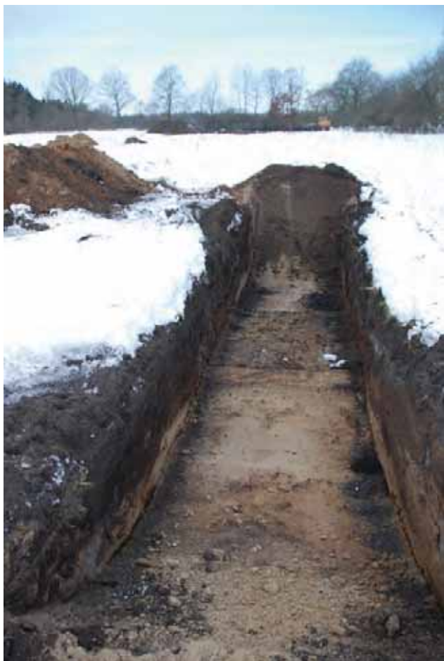
Sand dominates this site. A new pond would not retain water.
