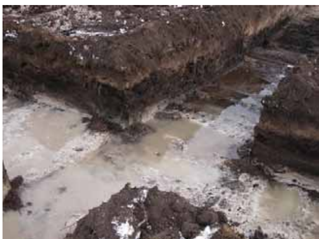
A typical test cross revealing different pedological layers (from top to bottom): organic brown top layer, light brown clay layer, dark brown clay layer with organic material and white clay bottom layer.
